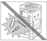
■ Be careful not to spill liquids or drop any foreign objects, such as paper clips or staples inside the machine. If a foreign object comes into contact with electrical parts inside the machine, it may cause a short circuit and result in a fire or electrical shock.
